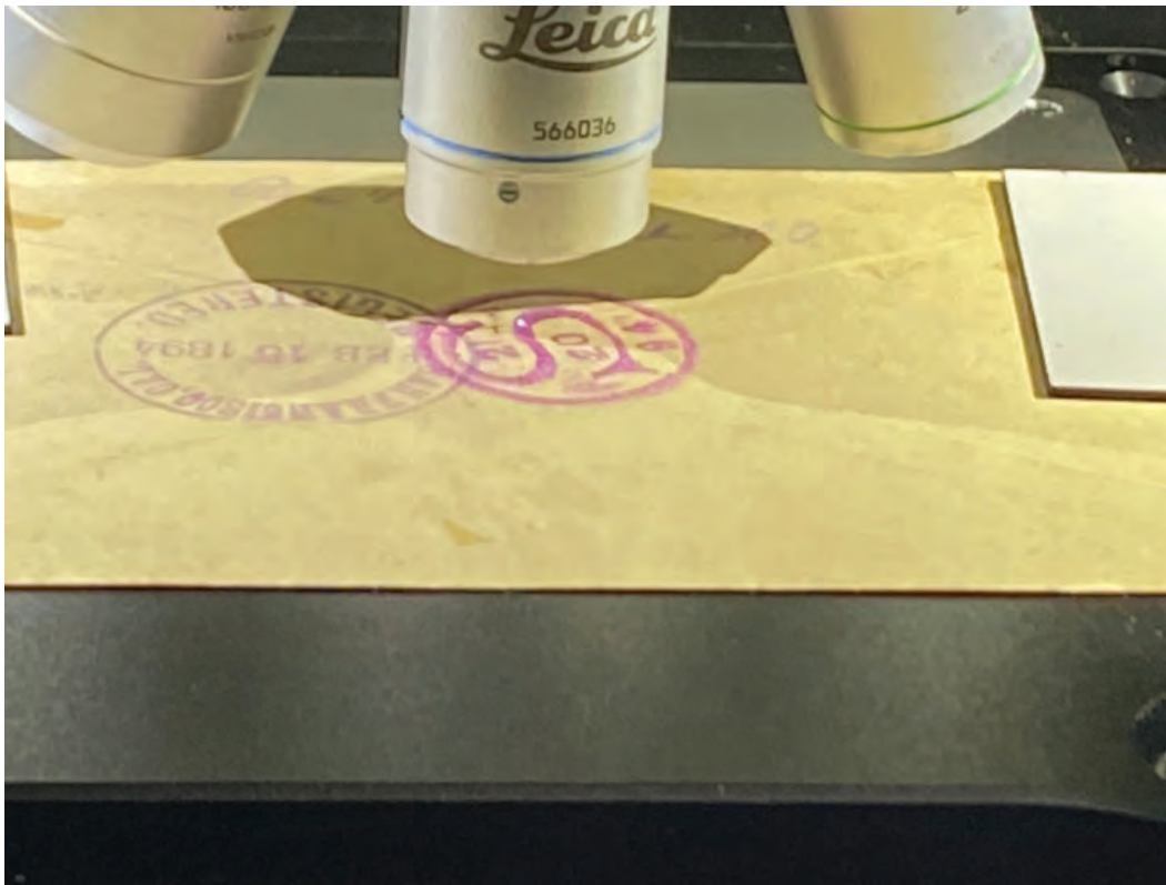
Figure 19. New York registry arrival CDS, Feb. 20, 1894, red-violet dye; the test point is on the internal “S” shown illuminated using the x50WLD microscope in the Renishaw Invia spectrometer.
