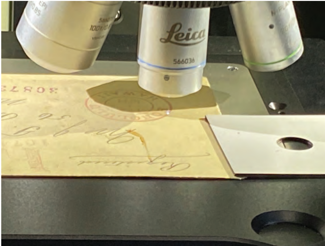
Figure 2. The Figure 1 cover front shown with the CDS circumference as the test point No. 1 is above Honolulu. It is shown illuminated in the Renishaw Invia spectrometer using the x50WLD microscope. The 457nm laser will be used.
