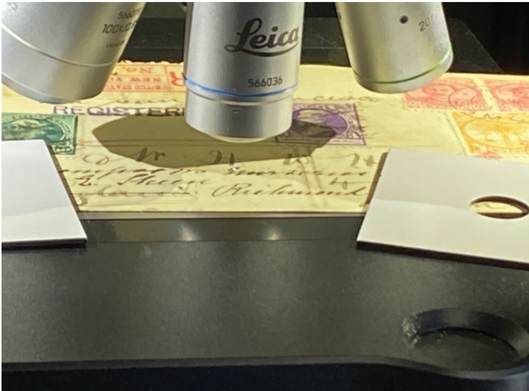
Figure 19. Sender's address script ink shown in the Renishaw Invia Raman spectrometer, illuminated using the x50WLD microscope. The 785nm laser will be used to obtain a Raman spectrum for compound matching.
