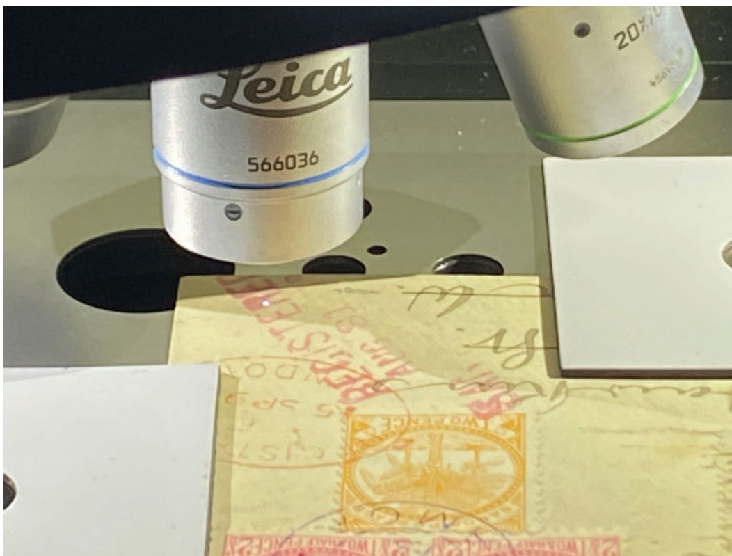
Figure 5, The Samoa-to-England cover is shown in the Renishaw Invia Raman spectrometer, with the test point in the “REGISTERED,” with red dye illuminated using the x50WLD microscope. The test point is the second “R” in the three-line hand stamp.
