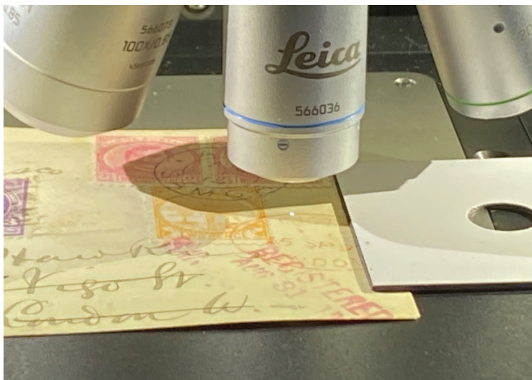
Figure 16, London, England, Sept. 15, 1894, registry oval datestamp shown illuminated using the x50LWD microscope in the Renishaw Invia Raman spectrometer. The 785nm laser will be used, the ink is anticipated to be Cinnabar or Mercury Sulfide a red inorganic ink.
