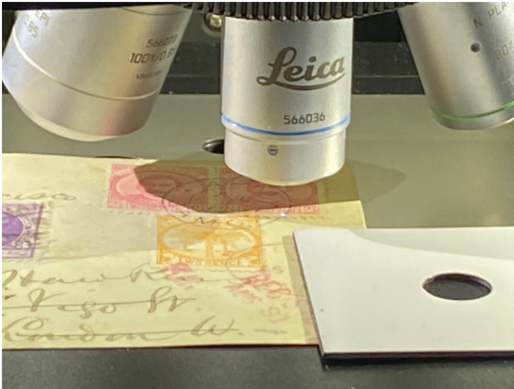
Figure 12. Samoa post office CDS shown in the Renishaw Invia spectrometer, illuminated with the x50WLD microscope. The outer circumference of the cancellation (on the stamp paper selvage) is the test point.
