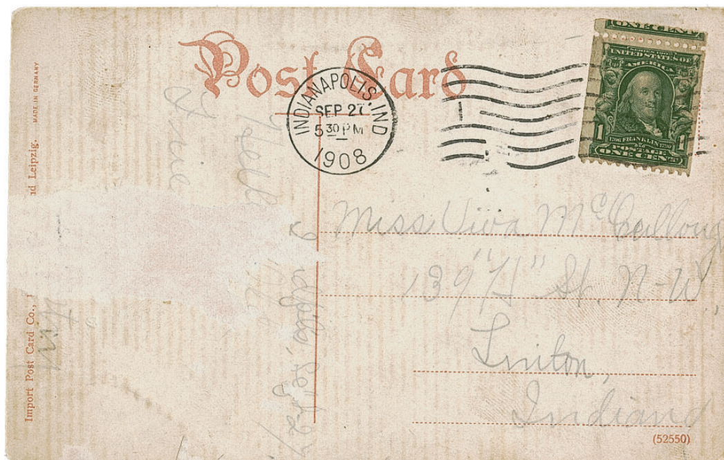
Figure 10 (above). A 1¢ vertical coil dispensed from a Parkhurst vending machine and dated Indianapolis, Sept. 27, 1908, during the 30-day trial period. The stamp shows the feeding mechanism misalignment that caused part of the adjoining stamp above to be torn off.
