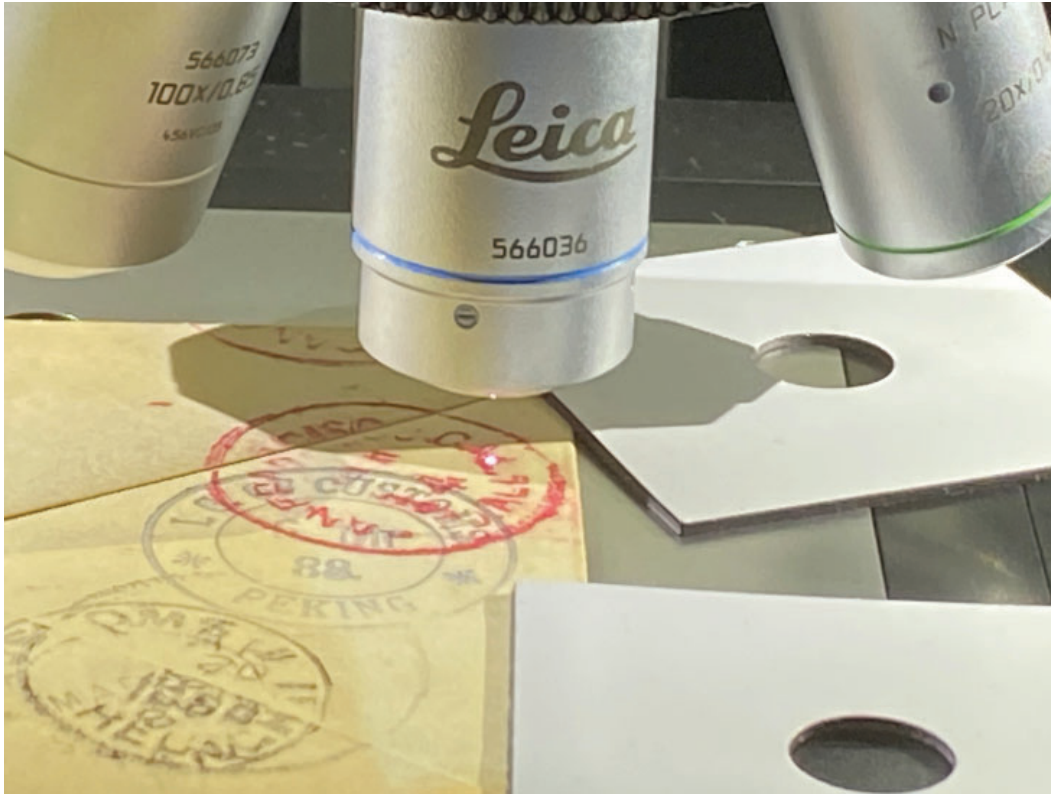
Figure 3. San Francisco transit CDS ink at test point No. 1, the “L” of CAL, as shown above illuminated using the x50WLD microscope.
