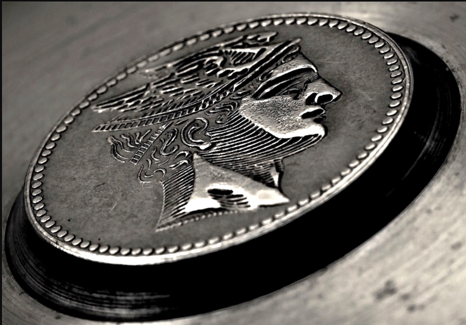
The matrix of the medallion die at its final stage (detail)
